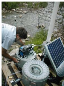
Fig. 4a. Servicing “R 2 D 2 ” the Teledyne ISCO automated water sampler located at the Rt 38A site. It collected 1-liter of water daily (4 am) and was serviced bi-monthly.
