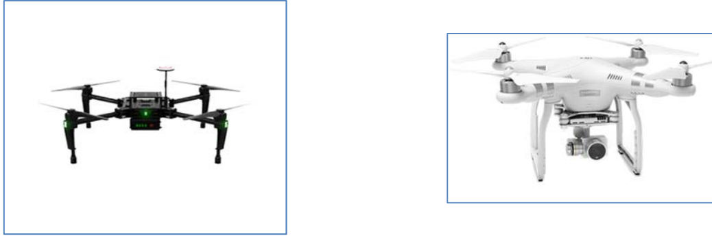
Fig. 3. The two drones used in this study, Matrice 100 (left) and Phantom 3 Advanced (right).
